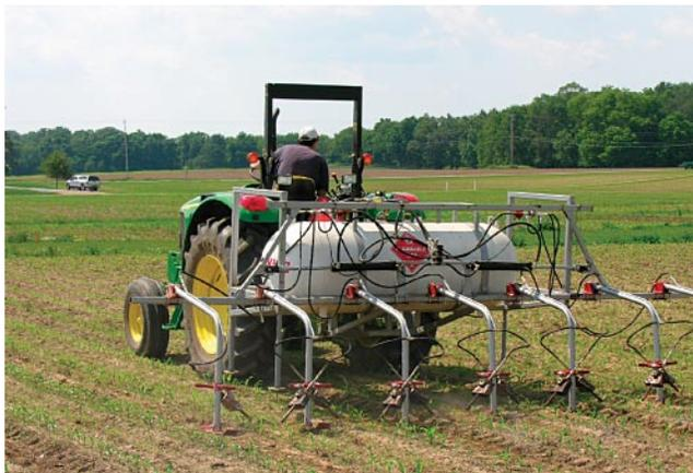
Fig. 3. Cross-flaming in organic corn. In this system of flaming, the torches are generally staggered while flaming so that each does not interfere with the flame from the opposite burner.
